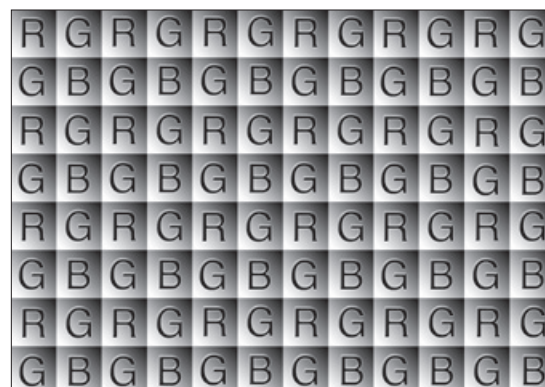
The Bayer Pattern, is an alternating four grid pattern.
