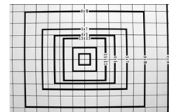
Photo 4 Taken with 50mm "normal" lens, note barrel distortion at edges.
